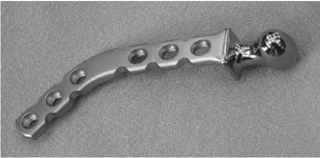
FIG. 7.388 Partial TMJ prosthesis.
